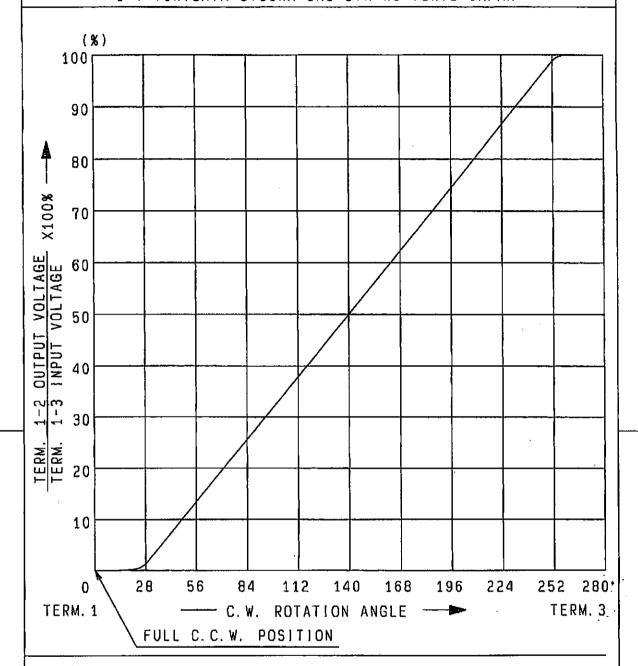
AT 140° C.W. SHAFT ROTATION FROM FULL C.C.W. POSITION VOLTAGE PERCENT SHALL FALL WITHIN THE LIMITS OF 40 $\sim$ 60 PERCENT.
